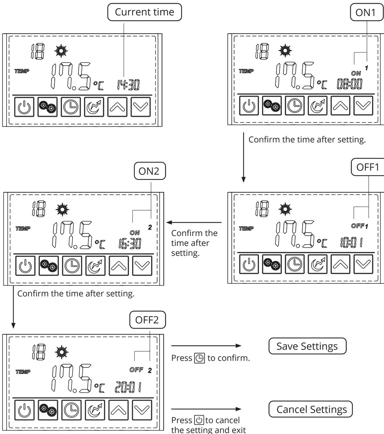
**NOTE:** Do not set the second timer to 00:00 ON and 00:00 OFF as the unit will commence heating at midnight every second night. To leave the second time off simply allow the timer setting to time-out after setting the first timer end time.
