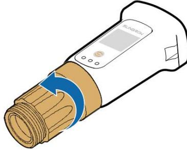
**Step 4** Thread the network cable through the swivel nut and gasket. Afterwards, route the cable into the opening of the sealing. Finally, insert the cable through the housing.
