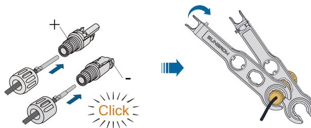
**Step 4** Check for polarity correctness.
