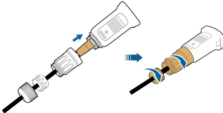
**Step 6** Remove the waterproof lid from the **COM1** terminal and install WiNet-S.
