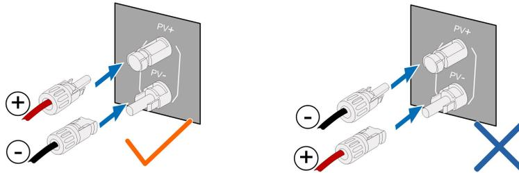
**Step 4** Seal the unused PV terminals with the terminal caps.
