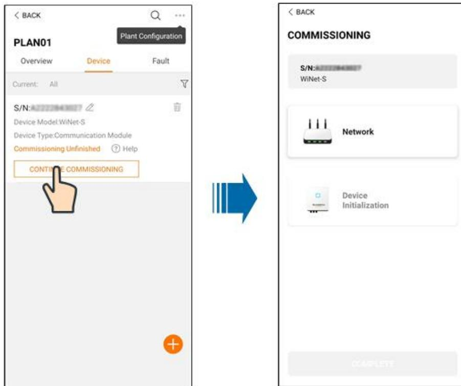
**Step 7** Tap **Network Configuration** to go to the **WLAN connection** interface. Tap the home network in the WLAN list, enter the password, and then tap **Confirm**.
