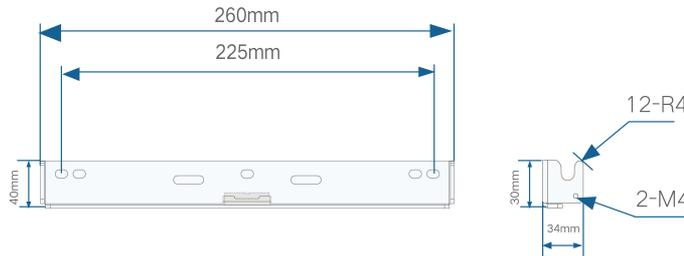
**figure 4-1** Dimensions of Mounting-bracket
