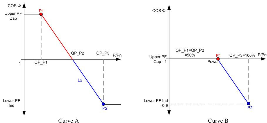
figure 7-18 Reactive Power Regulation Curve in Q(P) Mode
