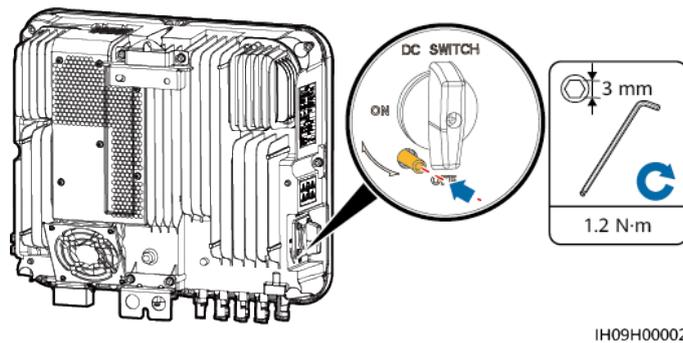
**Step 5** Install the inverter on the mounting bracket.
