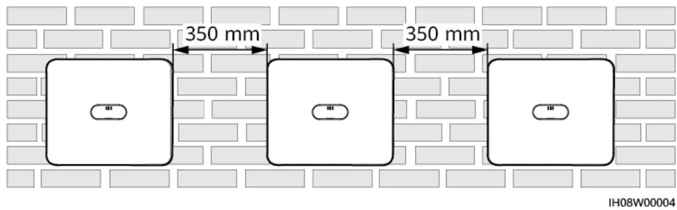
**Figure 4-4** Triangle installation mode (recommended)
