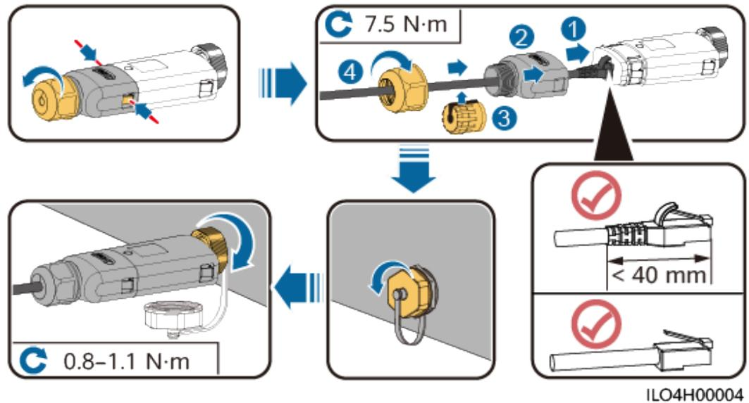
**Figure 5-35** Installing anti-theft components for the Smart Dongle
