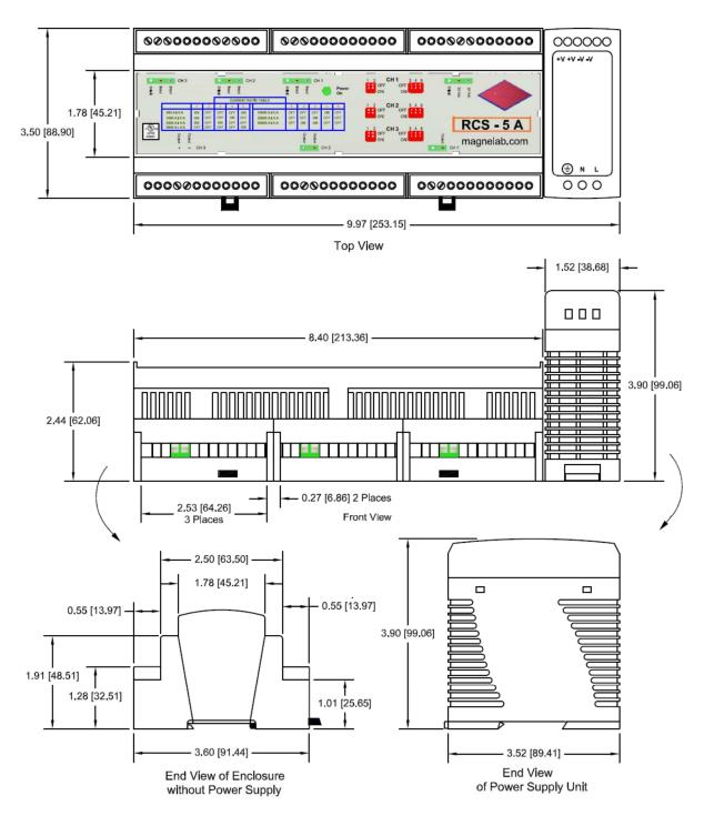
Dimensions are in Inches and Millimeters
