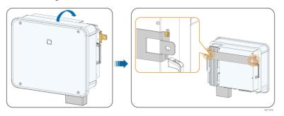
Step 3 Fix the inverter with screws.
