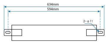
figure 4-1 Dimensions of Mounting-bracket
