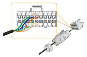
**Step 6** Pull the wires outward to check whether they are firmly installed.
