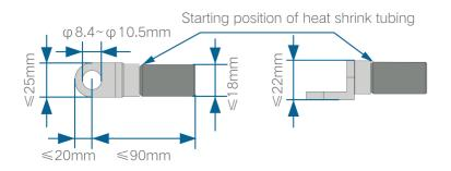
figure 5-3 Specifications of the Crimped OT/DT Terminal
