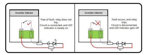
figure 5-5 Normally open contact
