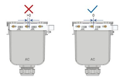
**Step 7** Gently pull the cable backwards to ensure firm connection, and fasten the swivel nut clockwise.
