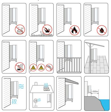
The inverter produces noise during operation, thus it is not recommended to install it in
