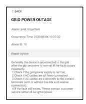
figure 7-9 Detailed Fault Alarm Information
