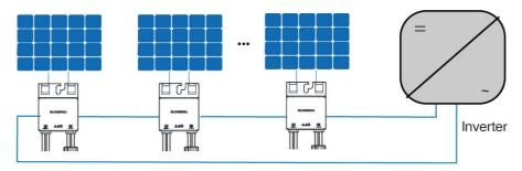
figure 4-2 Optimizers Configured for All PV Modules
