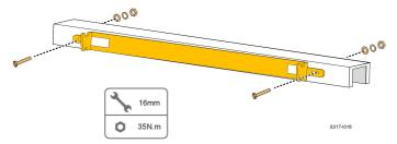
Step 4 Secure the steel u-channels to the pole with bolts and clamps.
