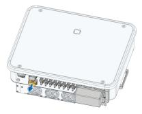
**Step 2** Insert the COM connector into **COM2** terminal on the bottom of the inverter until there is an audible click.
