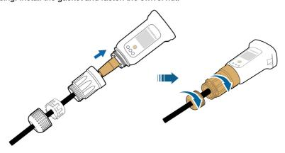
**Step 6** Remove the waterproof lid from the **COM1** terminal and install WiNet-S/WiNet-S2.
