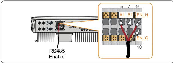
For the communication of battery that does not need to be enabled
