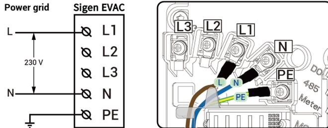
Three-phase five-wire system (L1/L2/L3/N/PE)
