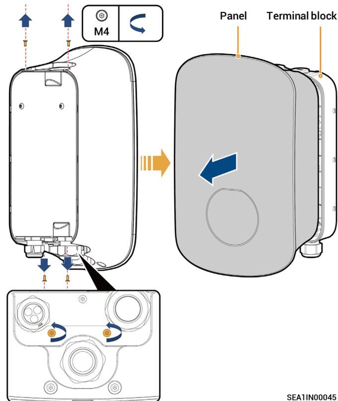
**3** Install and secure the terminal block.
