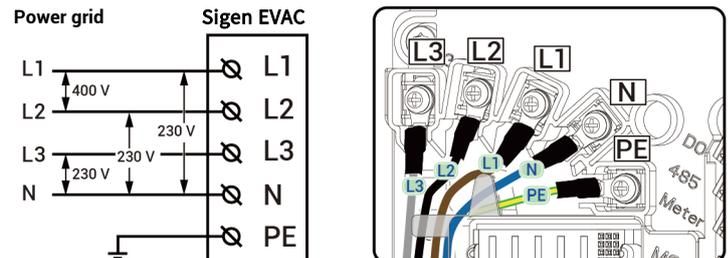
Three-phase four-wire system (L1/L2/L3/PE)
