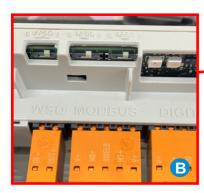
Set **MB1** switch **ON** for a single unit or last in chain **OFF** for all others
