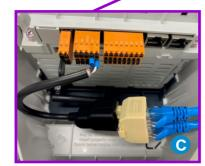
Chained Modbus for multiple units. See Fronius GEN24 installation manual for more details
