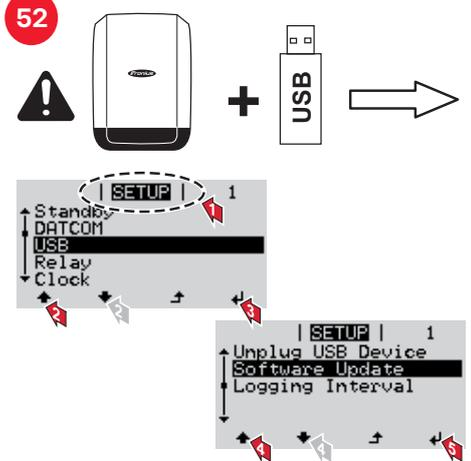
The display of the parameters to be configured depends on the selected device type
