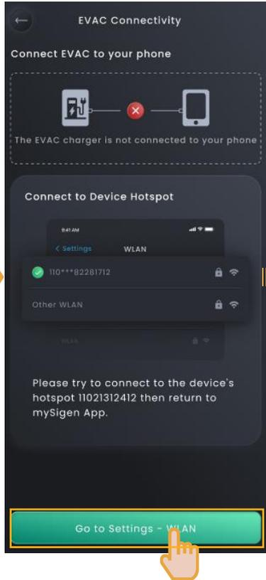
Connect to the equipment's WLAN hotspot. The hotspot is named as equipment SN and the passcode is given on the equipment label.
