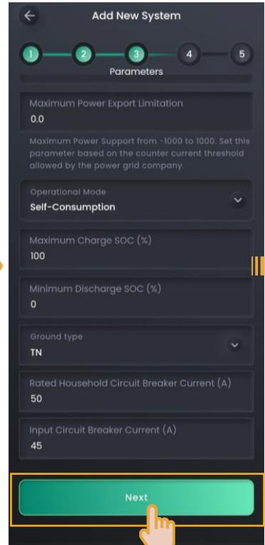
Set parameters as needed. Rated Household Circuit Breaker Current > Input Circuit Breaker Current > Default Output Charging Current
