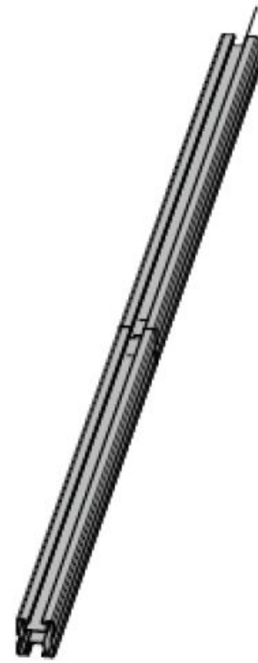
Fig 4.2.2C: Rails secured together via Proline joiner
