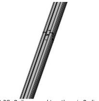
Fig 4.2.2C: Rails secured together via Proline joiner
