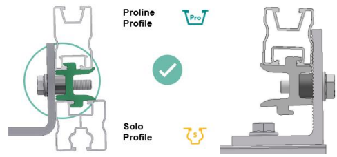
Fig 4.2.3A: Multi Adaptor fixing rail to fastener
