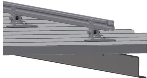
Fig 4.2.3B: Rail attachment to fasteners (substructure fixing)
