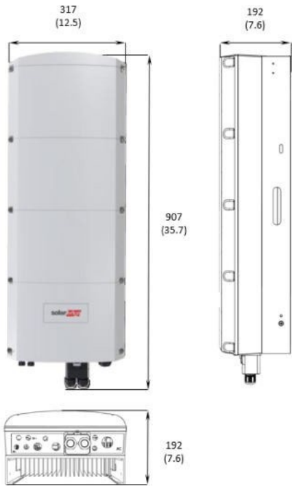
Figure 29: SolarEdge Home Hub Inverter - Three Phase: dimensions
