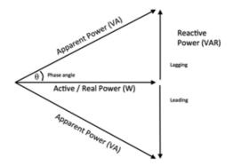
Power factor is defined as the ratio of the active power flowing to the load to the apparent power, and is expressed as a value between 0 and 1. The power factor can be leading or lagging, depending on whether the load is predominantly capacitive or inductive. Most residential installations would typically have a power factor of around 0.9 lagging, however commercial/industrial installations can often have power factors lower than this - in the range of 0.7 to 0.9.
