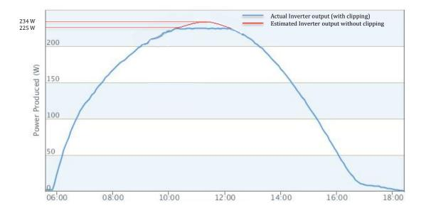
PV system designers can avoid clipping by sizing the microinverter such that it's output rating exceeds the highest expected output power from the solar module, taking into account the conversion efficiency of the inverter.
