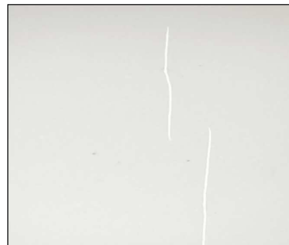
Cracks in 1s PVDF backsheet (KPf) after DH1000 + TC400 similar to cracks observed in the field
