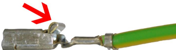
Figure 27: Latch on the earthing connector
