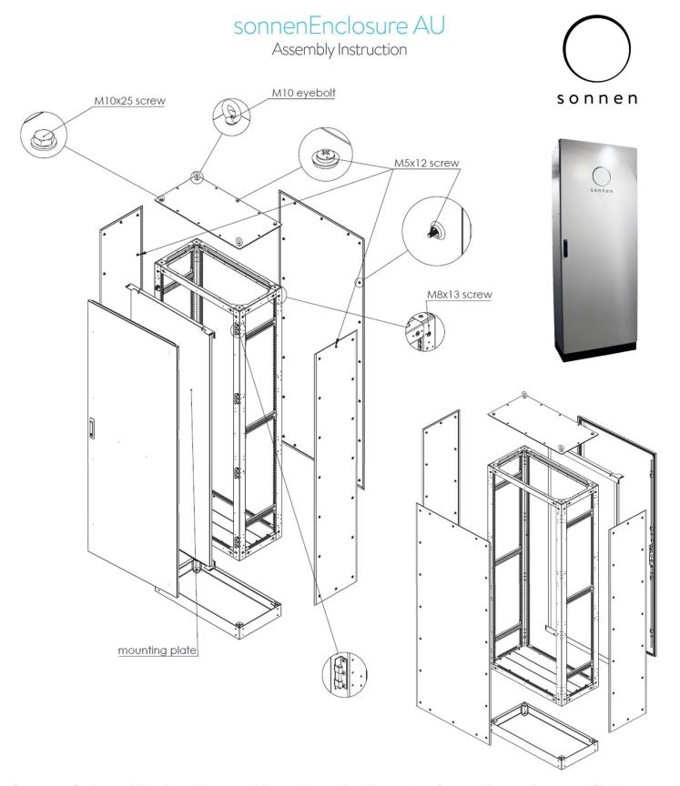
The sonnenEnclosure AU is shipped in a partial flat pack state. It will comprise of top and bottom frame sets. The inner vertical rails, internal mounting frame, side paneling and door. All screws and fixings are supplied.
