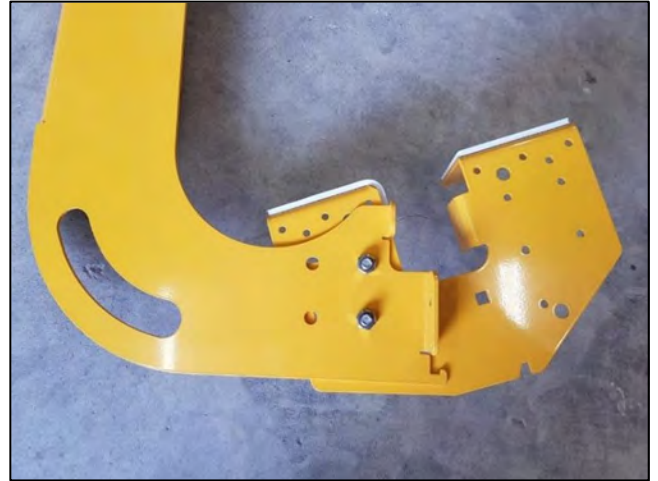
Picture shows bolts situated in forward bolt holes of re-roof bracket with rearward bolt holes beside them.
