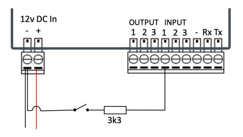
Figure 7.1 – Example circuit diagram using Input 1
