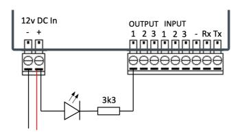
Figure 7.5 – Example circuit diagram for external LED
