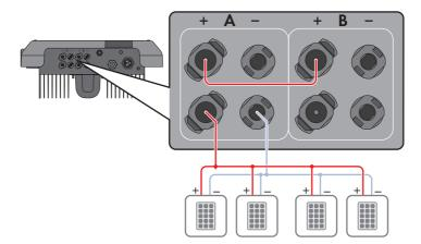
Figure 10: Connection overview for parallel connection of the DC inputs A and B
