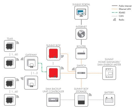
Figure 4: Design of system communication
