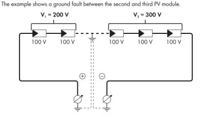
Test by Measuring the Insulation Resistance
