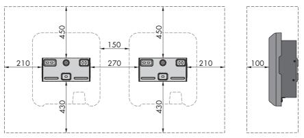
Figure 7: Recommended clearances(Dimensions in mm)
