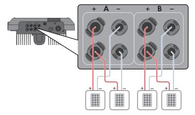
Figure 9: Connection overview for normal operation
