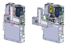
H) Drill the appropriate cutout on either the back or side of the unit or on both based on configurations. The rear entry can support the conduit with diameter of 1/2 in (13 mm) to 3/4 in (19 mm) while side entry can support the conduit with diameter of 1/2 in (13 mm) to 1-1/4 in (32 mm). Use the table to decide the cutout diameter and the conductor size required for line, neutral, and ground.
