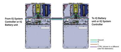
G ) Follow jacket stripping length and connect the control communication wires to 4-pin connectors as shown in the following image. Remove the resistor from control connectors from all the units except the one farthest from IQ System Controller in the daisy chain.
