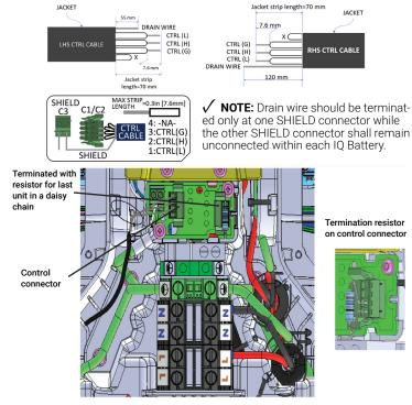
H) Route the conductors between conduit and terminal blocks using anchoring points as shown in the following figure:
