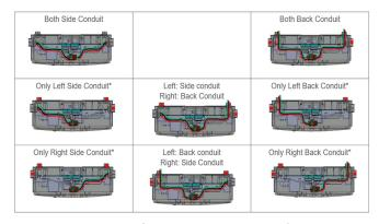
\* One side conduit configuration is supported only if system has only one IQ Battery or for the unit last in the daisy chain farthest from the IQ System Controller.
