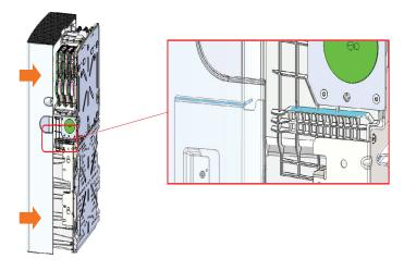
C ) Before releasing, pull out the lower edges while sliding in the cover and make sure the tabs are locked to the back plate as shown in the following figure:
