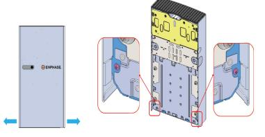
D) Push in the top portion of the cover as shown and make sure that the cover is locked in place as indicated.
