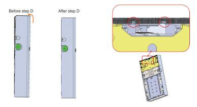
E) Fasten cover to the extension backplate using two M5 Phillips hex head screws (Torque to 3.1 N m)
