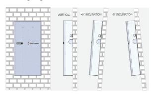
E) Make sure the mounting surface flatness is within 2 mm between boundary lines as shown in following image:
