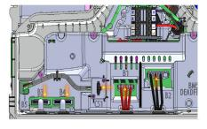
B ) Fasten (torque to 1.5 N m) the 11 captive screws at the wiring cover as shown. Use electric drive; do not use impact drives/impact drills.
