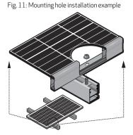
When installing using mounting holes, the frame of each panel must be supported by two rails of aluminium or galvanized steel suitable for the application and appropriate for the local environment. Observe the following procedures when using mounting holes:
