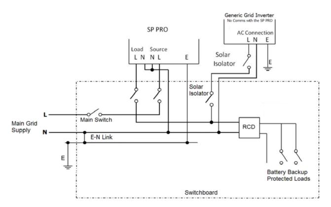
Line diagram for Generic AC coupling - Solar Hybrid System
