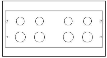
**2** - Cable entry is either from below or wall entry. Gland plates are inter changeable. Gland plates secure to the underside of unit base or to the inside of the mounting plate using four T25 Torx screws. **NOTE**: Any wiring via the rear gland plate (attached to mounting bracket) can be ruffed in before mounting the SP PRO.
