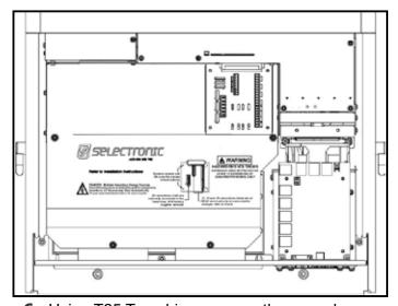
**6** - Using T25 Torx driver remove the cover by unscrewing two screws at the bottom of the SP PRO.
