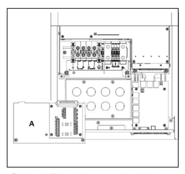
5 - Using the T20 torx driver remove the terminal cover and expansion card(A) by undoing the 2 screws.
