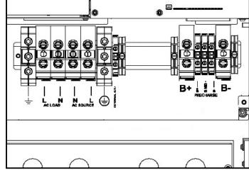
7- Undo five T20 Torx screws to remove terminal plate. Expansion card remains secured to SP PRO.
