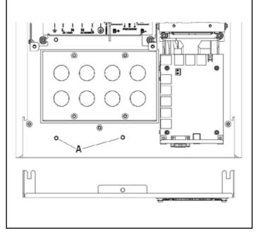
6 - The lower gland plate can be removed if required to give greater access to wiring terminals using T25 torx driver. NB, side screws need only be loosened. Secure the bottom of the SP PRO to the mounting plate with two M5 Torx screws. (A on above diagram)
