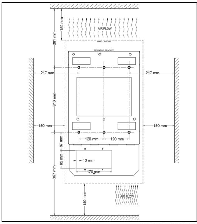
2 - Diagram previous page. Choose a suitable weight bearing and temperature resistant surface to mount the SP PRO. Mounting MUST be to solid timber studs, solid timber, brick, masonry or other load bearing wall. DO NOT mount directly to plaster. Max temperature is ambient +30 degrees C, max weight is 45 kg. The display of the SP PRO should be at eye level. There should be no obstructions to the clear passage of air. Use the 6 x M8 holes to mount the bracket.
