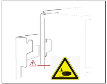
3 - Leave access cover (A) in place. Lift inverter from underneath whilst stabilising top. Inverter is top heavy and gloves must be worn. Mount the SP PRO on the mounting plate by first hooking the top of the inverter over the projections and lowering it into position. Care should be taken to observe Pinch Point warning.
