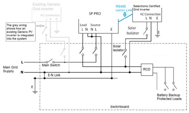
Line diagram for Managed AC coupling - Solar Hybrid (Grid Connected) System Diagram given as a reference only. Please ensure all wiring complies with relevant safety standards.
