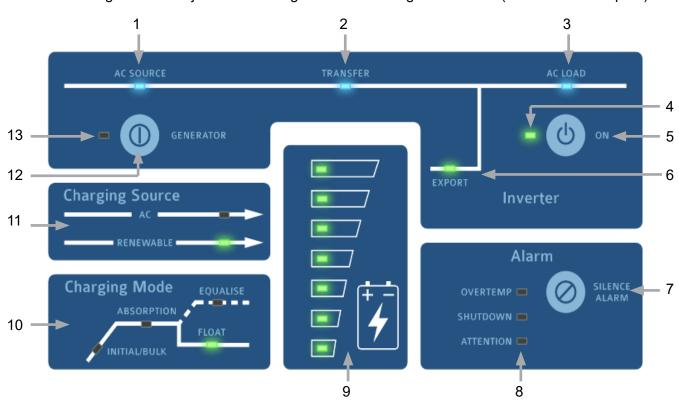
When illuminated, this shows the presence of AC supply voltage from either the mains grid or backup generator (when installed), whichever is applicable. This is powered directly from the incoming AC supply.
