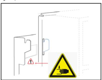
**5** - Mount the SP PRO on the mounting plate by first hooking the top of the inverter over the projections on the mounting plate and lowering it into position. Care should be taken to observe Pinch Point warning. Secure the bottom of the inverter to the mounting plate with two M6 bolts provided.
