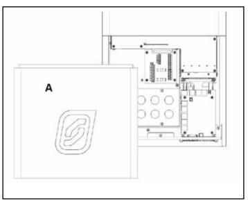
**4** - With a T25 torx driver, remove the access cover(A) by unscrewing the two M5 Torx screws at the bottom of the SP PRO.
