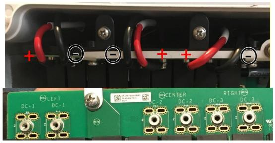
Figure 18: keep correct polarity
