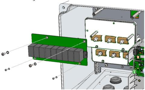
Figure 3: Removal of the DC SPD Board
