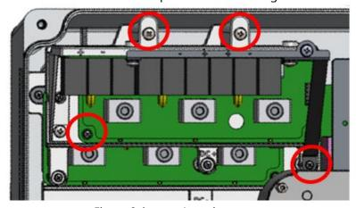
Figure 8: loosen 4 captive screws
