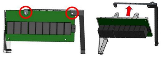
Figure 10: remove GND Bus Bar
