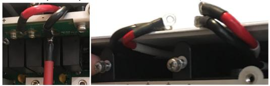
Figure 6: remove 6 screws
