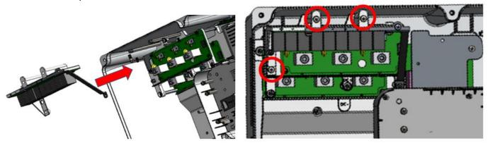
Figure 16: replace GND Bus Bar assembly tighten three M4 screws
