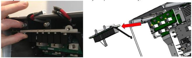
Figure 9: remove GND Bus Bar assembly
