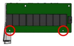
Figure 14: place SPD Board onto DC SPD holder
