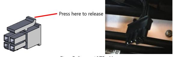
Figure 7: disconnect NTC cable
