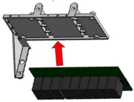
Figure 13: place SPD Board into the DC SPD Holder
