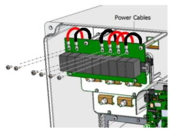
Figure 2: Power Cable of DC SPD Board
