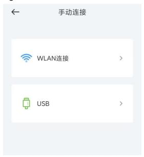
Select WLAN and connect to the corresponding WLAN in the WLAN connection list of the APP. The initial name of the WLAN hotspot is solar inverter SN, and the initial password is Changeme.
