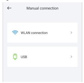
Select WLAN and connect the SmartLogger1000A or SmartLogger3000 to the corresponding WLAN in the WLAN connection list of the APP. The initial name of the WLAN is Logger\_SN bar code, and the initial password is Changeme.
