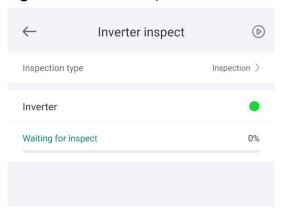
**Step 2** Choose **Inspection type**, tap in the upper-right corner of the screen to start solar inverter inspection.
