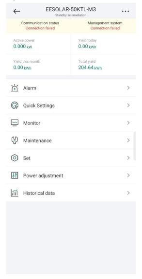
**Step 2** Tap **Alarm** or **Device Monitoring** to view active alarms, historical alarms, and running information of the solar inverters.
