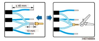
Figure 5-24 Assembling a signal connector (single inverter)
