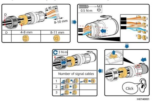
Figure 5-25 Assembling a signal connector (inverter cascading)
