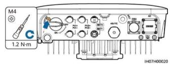
**Step 5** Install the inverter on the mounting bracket.
