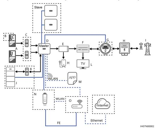
Figure 2-2 Smart solar inverter cascading scenario (dashed boxes indicate optional configuration)
