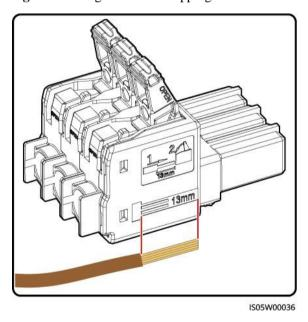
**Step 2** Connect the AC connector to the AC output port.
