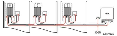
**Step 4** Set the DC switch to OFF and check whether the connector or DC cable between the possible faulty PV modules and the corresponding optimizers, or those between the adjacent PV modules and the corresponding optimizers are damaged.
